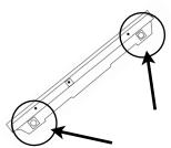
Press the buttons on the bottom to release the back plate from the panel face
