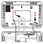
Secure the back plate to the wall, then loop the hang strap over the strain relief hook (1) Run the antenna through the hole (2)
