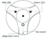
the glass break detector. The Glass Break Detector should first acknowledge the detection of a thud sound by illuminating the green LED and then illuminate the red LED when the unit detects the crash portion of the glass breaking sound.
