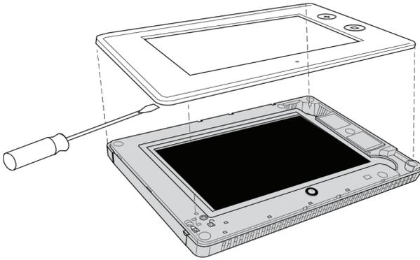
2. Remove the door-lock screw from the UNLOCK position on the right.
