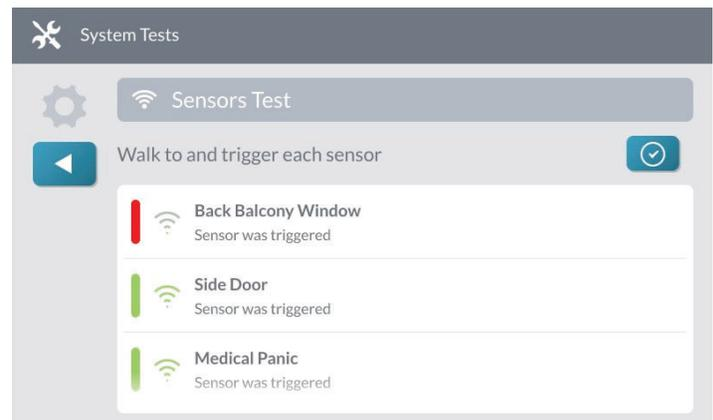
When tests are successful, a **GREEN** bar appears to the left of the test name. This indicates the sensor is operating and the wireless signal strength was good.
