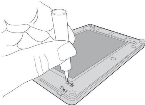
3. Install the screw into the LOCK position on the left. This locks the hinged door on the GC3e Control Panel.
